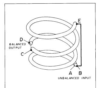
fig. 1. The 1:1 broadband coaxial balun. Actual transformer consists of seven turns closewound (3½ turns either side of the output) of RG-8X coax approximately 4 inches (100 mm) diameter. Center conductor in upper winding is not used.
