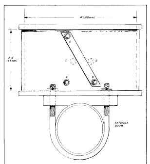
fig. 2. Physical layout of cylindrical balun housing. Output termination points C and D are located on the opposite side of the container. Top and bottom covers are epoxied in place. B-E jumper is mounted on outside of housing to identify shield side of input.
